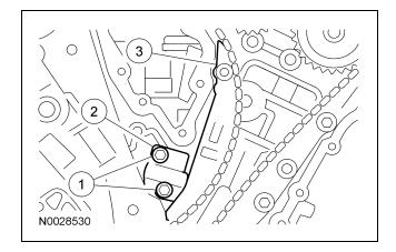
13. Remove the LH timing chain and timing chain guide.
