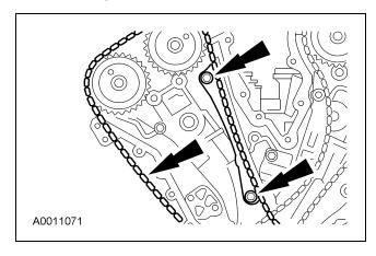
10. Rotate the crankcase clockwise 600 degrees (1-2/3 turns) to position the crankcase keyway in the 11 o'clock position. This will position the LH camshafts in the neutral position.
