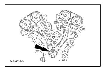
6. Rotate the crankshaft clockwise 120 degrees to the 3 o'clock position to locate the RH camshafts in the neutral position.
