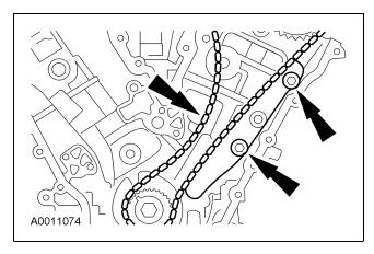
14. Remove the damper bolt and the crankshaft sprocket.
