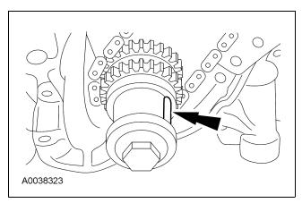
11. Verify that the RH camshafts are correctly positioned.
