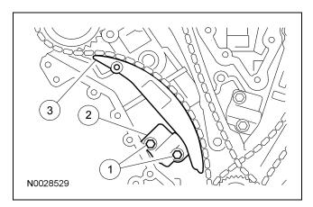
9. Remove the bolts, RH timing chain guide and the timing chain.
