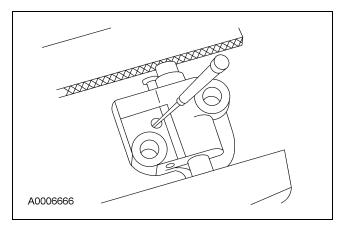
4. CAUTION: During tensioner compression, do not release the ratchet stem until the tensioner piston is fully bottomed in its bore or damage to the ratchet stem will result.
